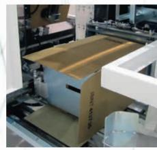
Positive motorized. Automatic cartons In feed conveyor with different loading Blank picking system provided with motor. opening and products insertion.
