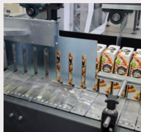
Automatic pushing system allows the products to be gathered in multipacks or pushed single
