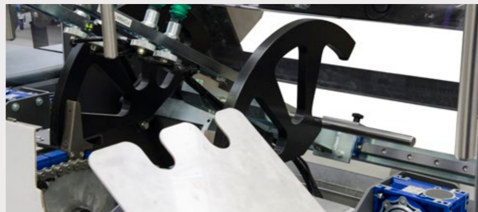
Carton loading and opening stations are mounted on sliding linear guides for a further accessibility during the maintenance operations.
