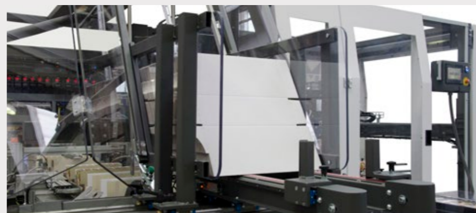
Wide carton blanks magazine for different sizes, quick and easy change of format.
