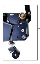
The access slot allows for ease of threading the head. The one way brass roller (larger brass roller) requires no maintenance and has adjustments to assist in tape application.
