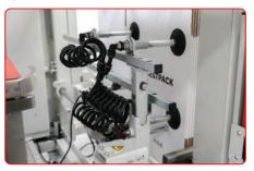
ROVED PICK UP ARM DESIGN Quickly adjust pick-up arms for carton size changes, boosting machine throughput and efficiency.
