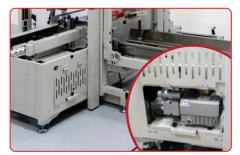
**VACUUM PUMP GUARD** Hide your vacuum pump to remove an additional safety hazard. Can easily slide out for maintenance.
