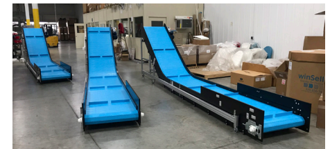
High impact belt with continuous side walls and abrasion resistance.
