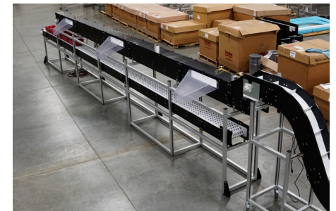
Multi-stack conveyor solution with three sort/divert stations.
